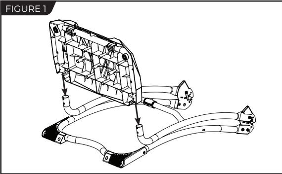
**IMPORTANT:** Do not fully tighten the bolts until all the bolts have been screwed in and the platform is properly aligned.
