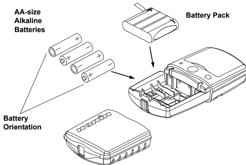
Figure 3: Installing Batteries
