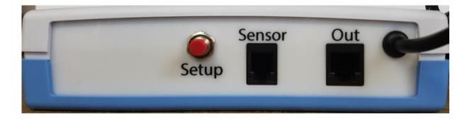
Insert the connector of the supplied sensor into the sensor socket, the connector will click in. The sensor connector does not require a strong force to be inserted
