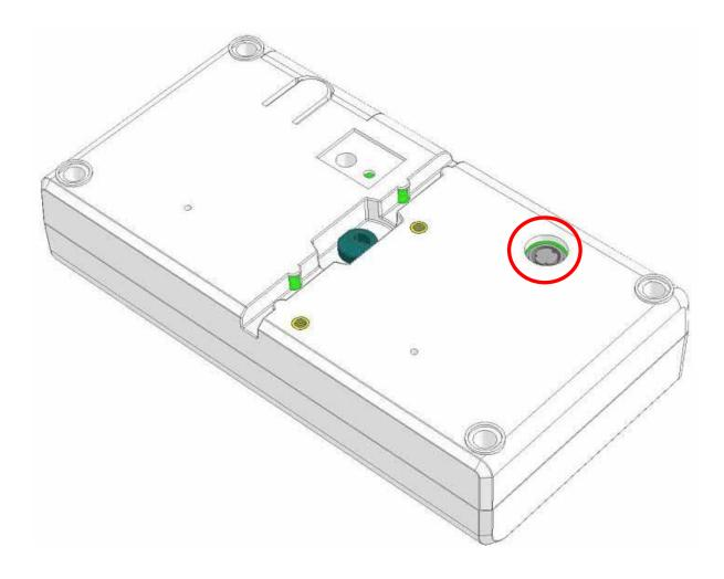
Insert the HM-201D data cable into the socket of the indicator before use.
