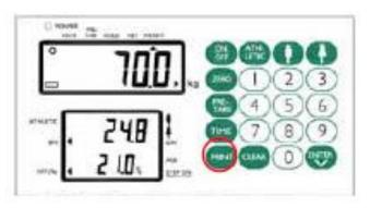
7. Press ENTER, and a flashing arrow will appear in the lower right corner. When this displays you can stand on the scale.
