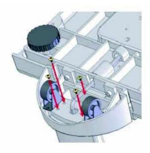
2. Holding both base and column, turn the scale over and secure with screws, as shown in the graphic on the left.
