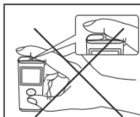
Inadequate contact between the electrodes and your finger.
