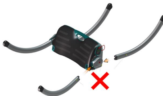
Incorrect assembly (do NOT mount the legs at first)
