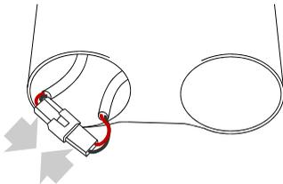
Then sit the connection inside one of the supplied bungs and insert the bung into the bottom of the downtube.
