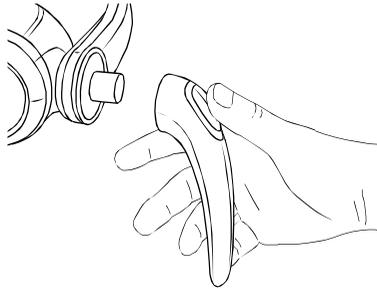
After use, turn off at the lighthead with the sensor or switch. Where applicable, also turn off the light at the power-supply via the wall mounted module or switched fused spur.
