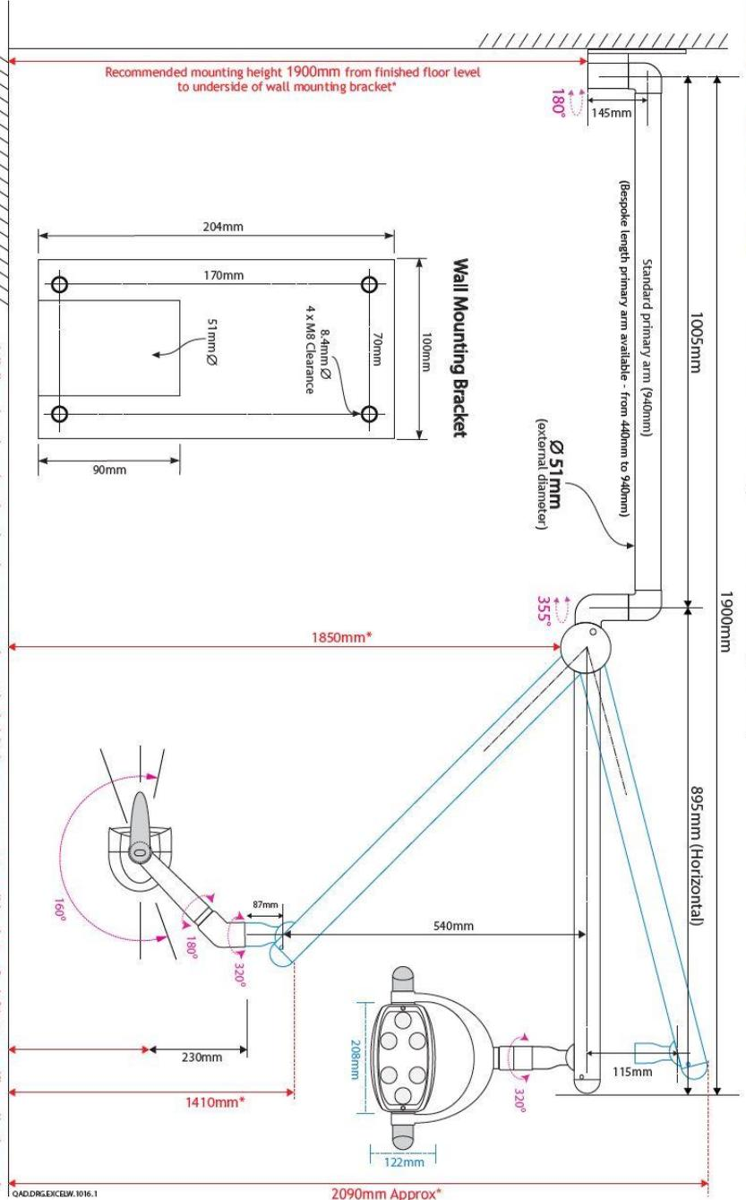
\*All dimensions shown in red are based on a suggested mounting height. (See measurement to wall bracket on far left). For specific applications and environments, the mounting bracket should be installed at a height so that, when fitted, the lighthead is as near to the required position as possible. Actual location should be dependent on intended use and desired reach. Common sense should always prevail.
